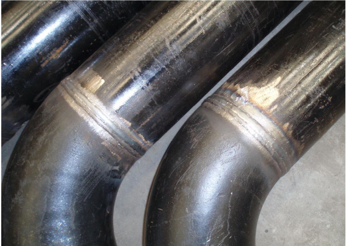
Liam Bagley- Ø300 pipe welding on Corus
